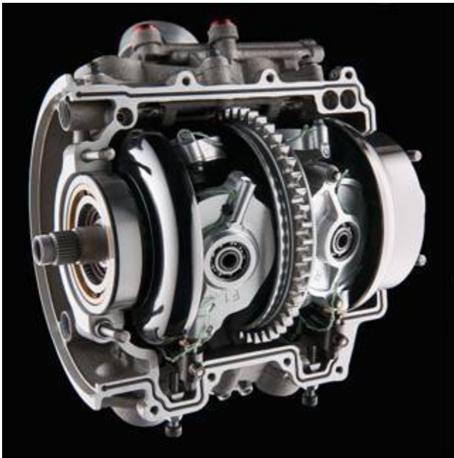
Figure 10: The Torotrak Full-Toroidal Twin Cavity Variator Configured for KERS Applications
